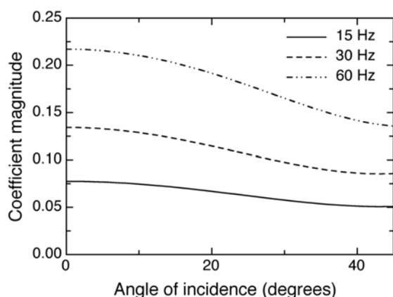
Figure 6: Composite reflection coefficient generated for interval (3.75 to 3.78 km) for three frequencies (15 Hz, 30 Hz and 60 Hz, in red, blue and black respectively).
