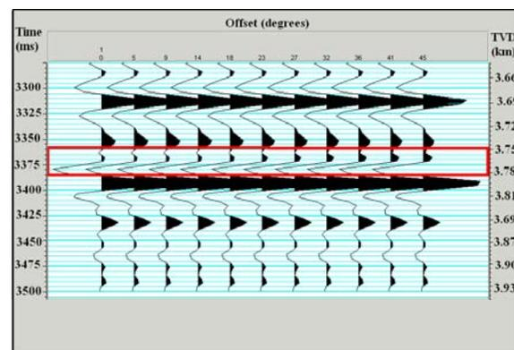
Figure 5: Synthetic seismic response generated with Zoeppritz approximation and, a 30Hz Ricker wavelet to a maximum of 45 degree offset. The equation assumes brine saturation and the red box corresponds to the lowest depth interval on the well log (3.75 to 3.78 km).
