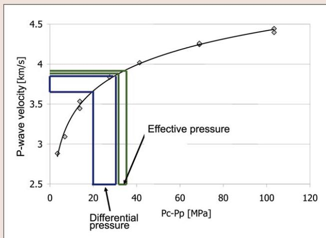
Figure 9. Compressional-wave velocity for a clastic sediment ( $\phi=13\%$ ) as a function of stress, using differential and effective pressure laws. In this case, for  $n=1$ , a change in  $P_p$  of 10 MPa leads to a change of 3.65 km/s to 3.85 km/s in  $V_p$  (blue outline). In contrast, for an  $n=0.5$ , a decreasing pore pressure of 10 MPa, will result in an effective pressure change of 5 MPa and produce a much smaller change in  $V_p$ : from 3.9 km/s to 3.95 km/s (green outline).
