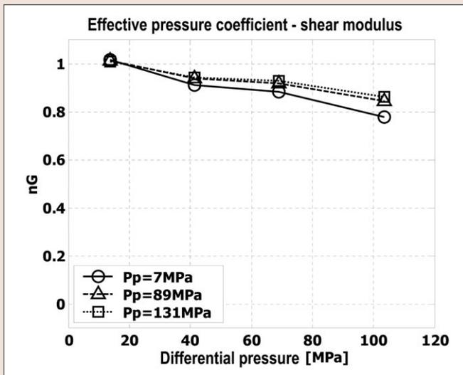
Figure 8. Effective pressure coefficients for brine-saturated shear moduli ( $nG$ ) as function of differential pressure for different pore pressures. All brine-saturated data have been normalized to the properties of brine at  $P_p=3.9$  MPa (1000 psi).
