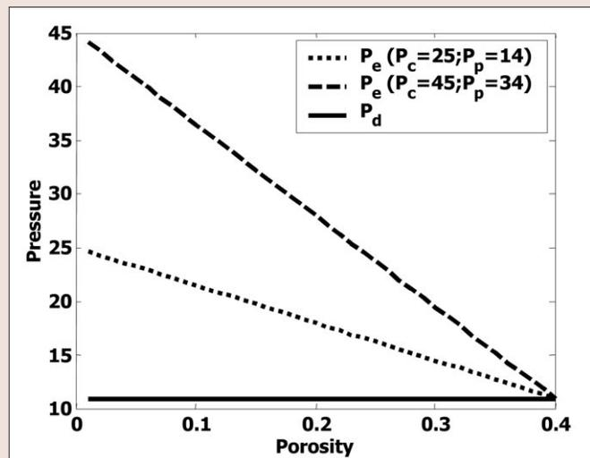
Figure 2. Effective pressure as function of the porosity. For two in-situ conditions ( $P_c=25$  MPa,  $P_p=14$  MPa;  $P_c=45$  MPa,  $P_p=34$  MPa) the differential pressure is constant ( $P_d=11$  MPa) as function of porosity; with a decrease of porosity, the effective pressure increases depending on  $P_c$  and  $P_p$ .
