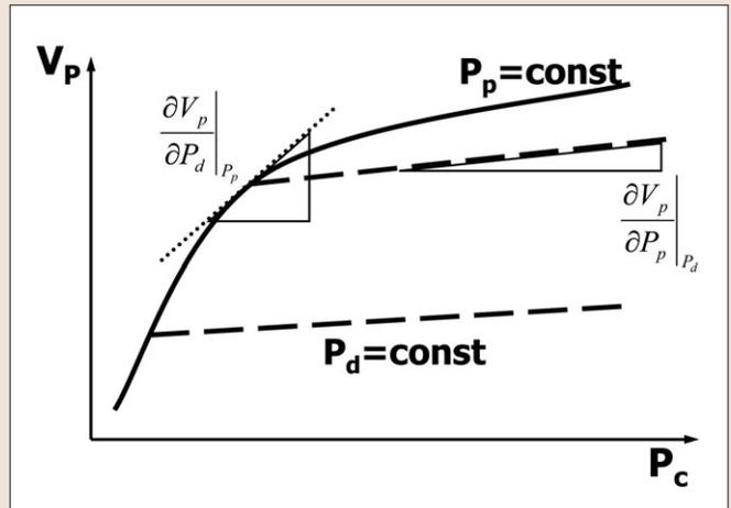
Figure 3. Schematic behavior of compressional wave velocity ( $V_p$ ). The two derived quantities for constant differential and constant pore pressure are indicated.
