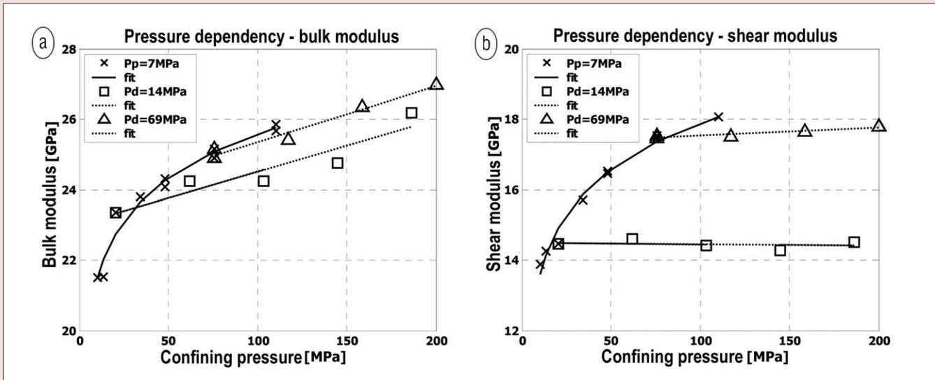
Figure 6. Pressure dependency for normalized saturated bulk (a) and shear modulus (b) as function of confining pressure, for constant pore pressure ( $P_p=7$  MPa), and constant differential pressure ( $P_d=14$  MPa and 69 MPa). All brine-saturated data have been normalized to the properties of brine at  $P_p=3.9$  MPa (1000 psi).
