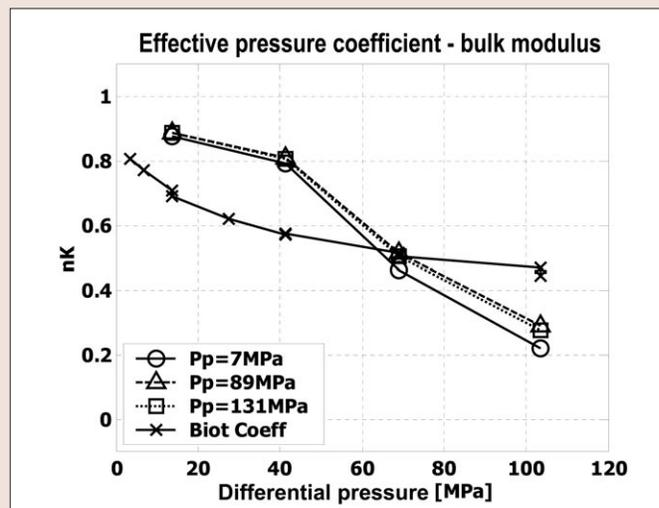
Figure 7. Effective pressure coefficients for brine-saturated bulk moduli ( $nK$ ) as function of differential pressure for different pore pressures in comparison to the Biot-Willis coefficient derived from the dry measurements. All brine-saturated data have been normalized to the properties of brine at  $P_p=3.9$  MPa (1000 psi).
