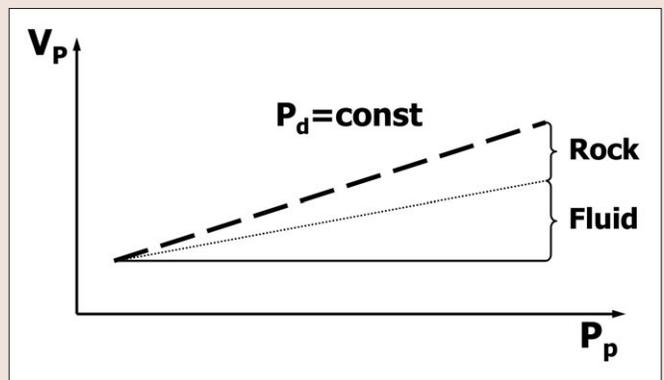
Figure 4. Compressional wave velocity ( $V_p$ ) as function of pore pressure. The contributions from changing fluid properties and rock properties are indicated.
