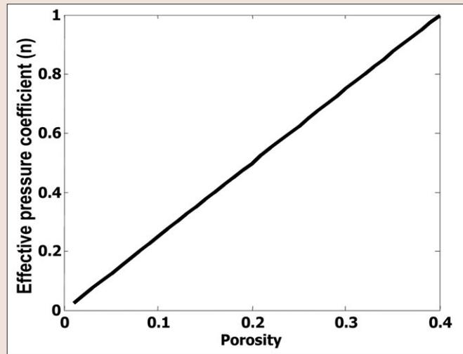
Figure 1. The effective pressure coefficient for bulk modulus as function of porosity. The critical porosity concept is applied to calculate the dry bulk modulus, which is then applied through the Biot-Willis theory.
