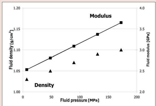
Figure 5. Changes in brine density and modulus as function of the pore pressure (triangles indicate density - right axis, squares indicate modulus - left axis).
