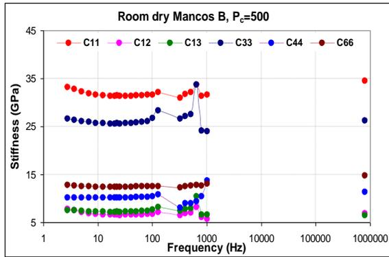
Figure 4: Estimated stiffness for room dry sample at  $P_d=500$ psi as a function of frequency from 2Hz-800 KHz.
