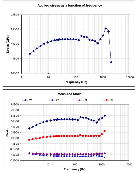
Figure 3: a) Applied stress for Mancos Shale at  $\theta=90^\circ$ , b) Measured strain on Mancos B Shale at  $\theta=90^\circ$ .
