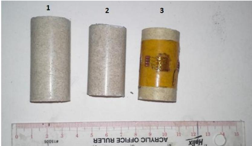
Figure 3: Prepared Fox Hill Sandstone samples, 1-2) coated with a thin layer of epoxy 2) coated with a thin layer of epoxy 3) strain gages have been glued to the sample
