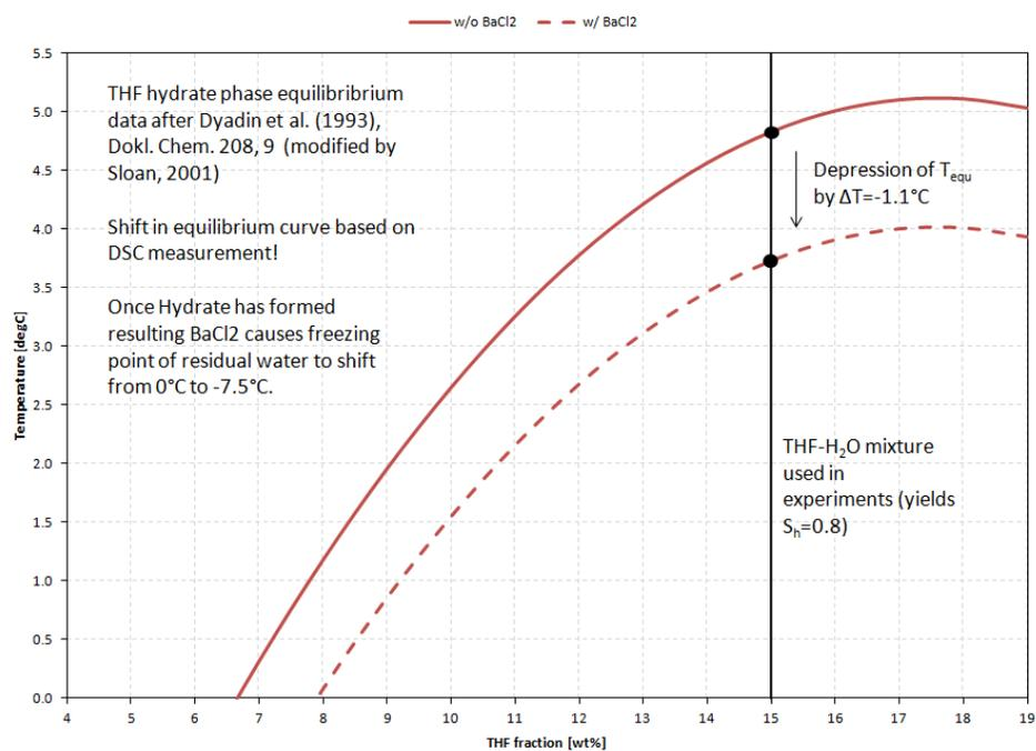
Figure 8. Depression of the hydrate equilibrium temperature associated with BaCl<sub>2</sub> in solution.
