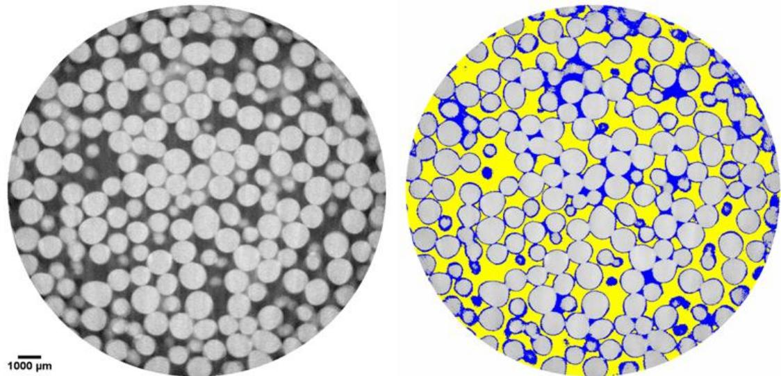
Figure 11. Calculation of water saturation in sample “glass\_beads+water3”, left: raw MXCT image, right: processed image with air-filled porosity shown in yellow and water-filled porosity shown in blue.
