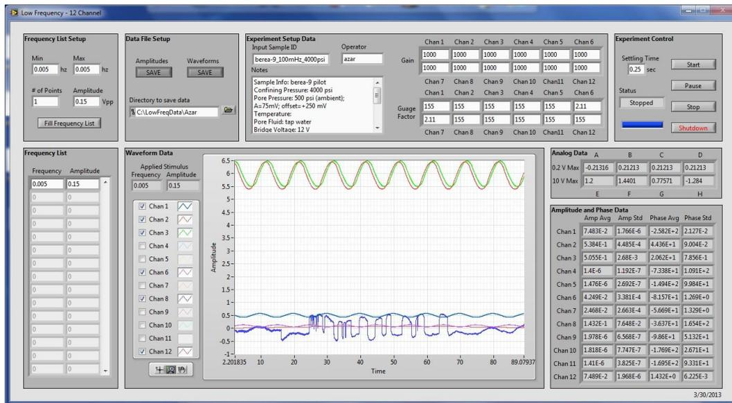
Figure 2. Labview screen controlling data acquisition.
