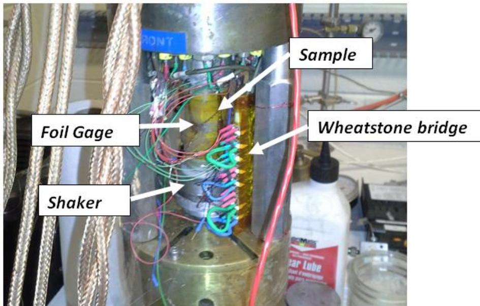
Figure 6. Sample in the low frequency device.
