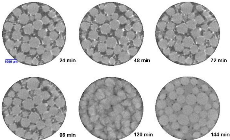
Figure 9. Micro X-ray CT images of dissociating THF hydrate in a glass bead sample
