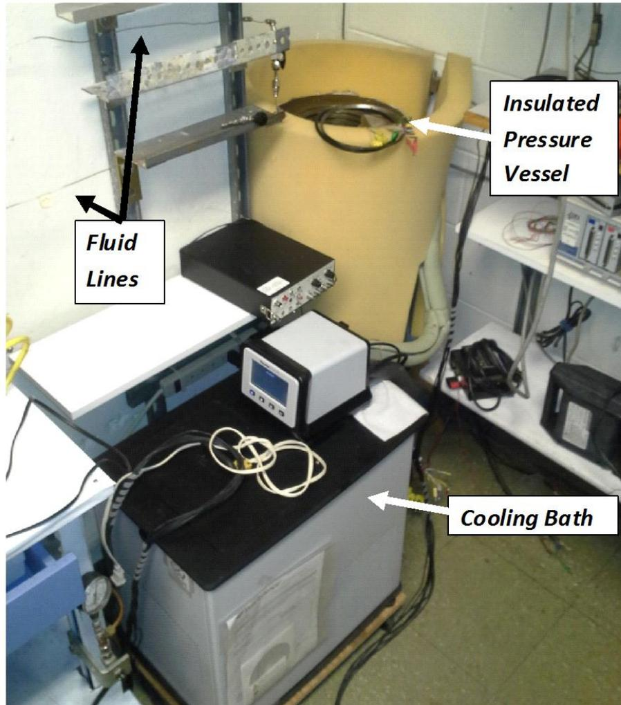
Figure 1: Insulated pressure vessel and cooling bath. This setup has been tested and temperatures can be controlled below freezing conditions.
