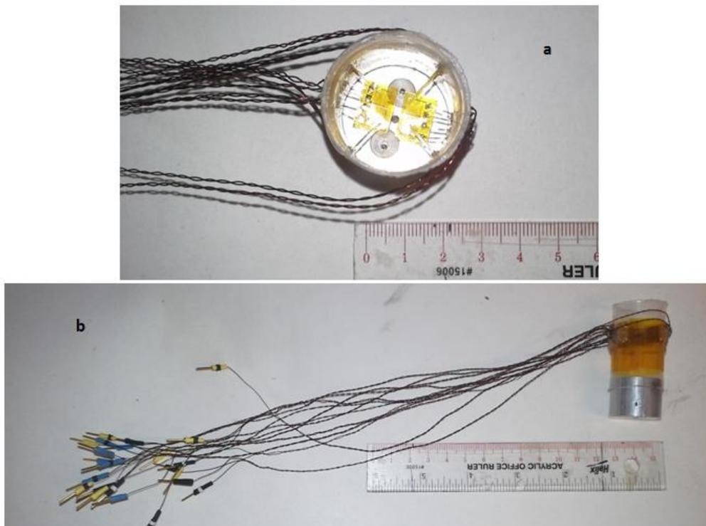
Figure 4. a) Sample holder for pure THF hydrate low frequency measurements (top view)
