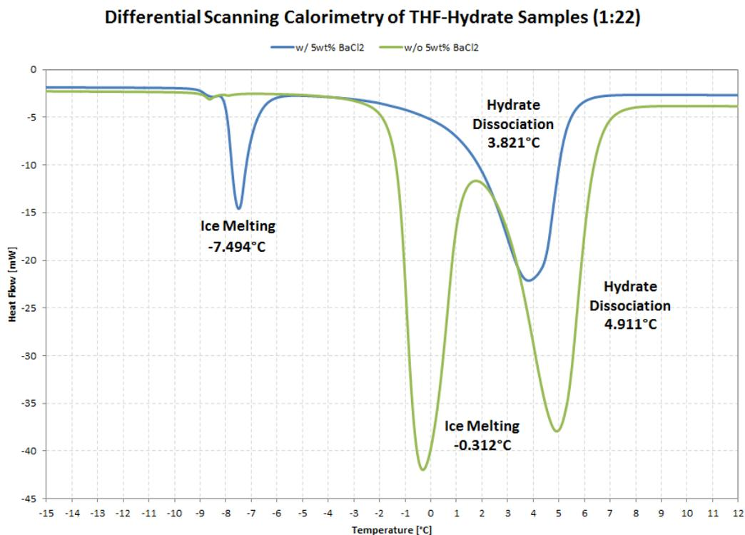
Figure 7. Disassociation of THF hydrate with BaCl<sub>2</sub> (blue line) and without BaCl<sub>2</sub> (green line) as indicated by Differential Scanning Calorimetry (DSC).
