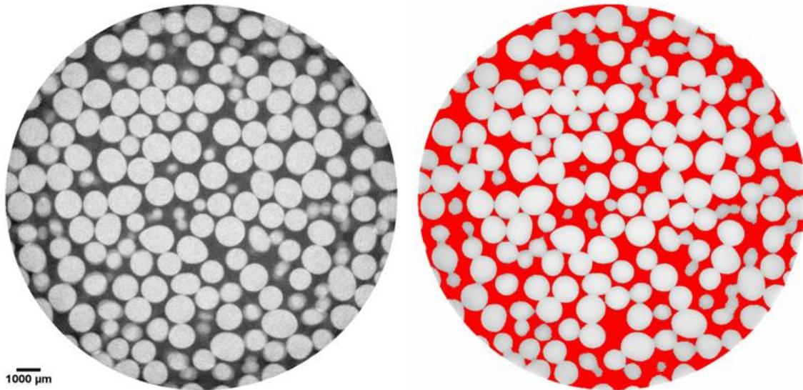
Figure 10. Porosity calculation in sample “dry\_glass\_beads\_4”, left: raw MXCT image, right: processed image with porosity shown in red
